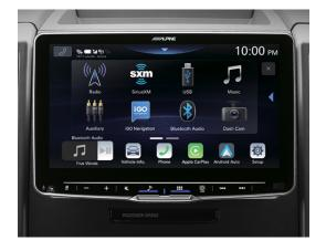
**Navigation Features** – After plugging the KTX-NS01 into the Alpine radio, a navigation app will appear on the home screen, providing instant access to the HERE map database with maps of the United States and Canada. Voice prompts for turn-by-turn directions are also available and are projected from the vehicle's sound system.
